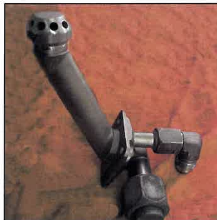
Low-Btu Nozzle. Stock steam injection nozzle designed for conventional NOx reduction and natural gas fuel injection, with ten 0.210-inch diameter holes.
