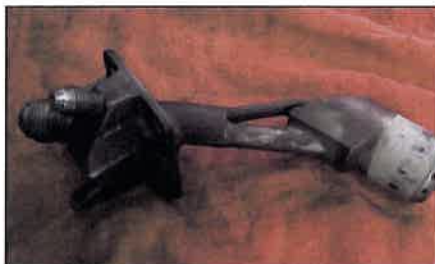
Dual Fuel Nozzle. Stock dual fuel nozzle designed to operate on natural gas and distillate. Nozzle tip has twelve 0.100-inch diameter holes.
