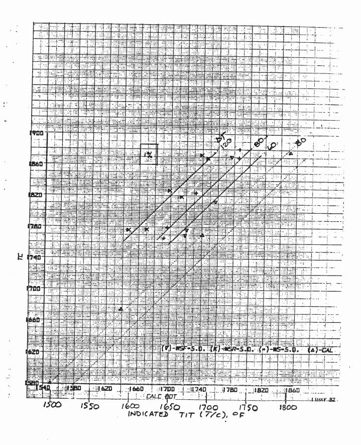
Figure 8 501 steam injection test data -  $T_C$  vs calc BOT for  $W_S$ =5.0
