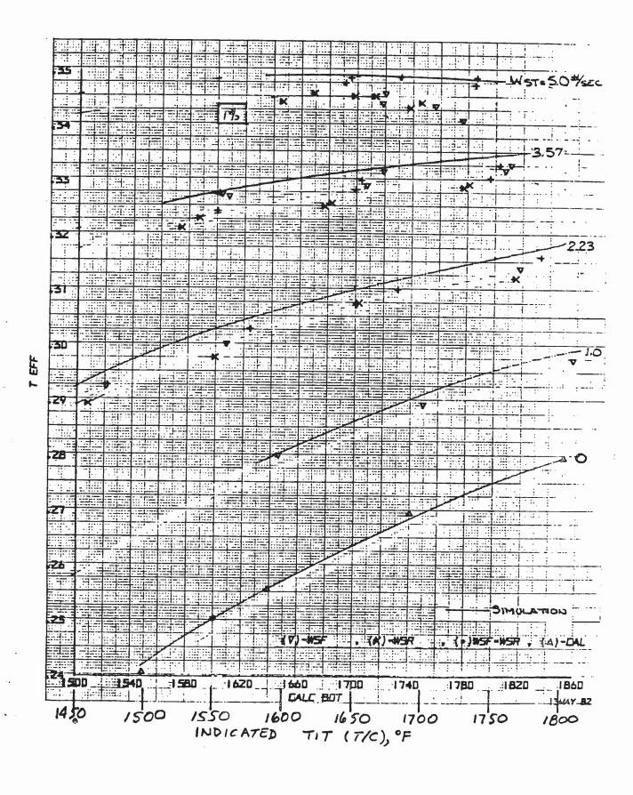
Figure 3 501 steam injection test data - Thermal Efficiency vs calc BOT
