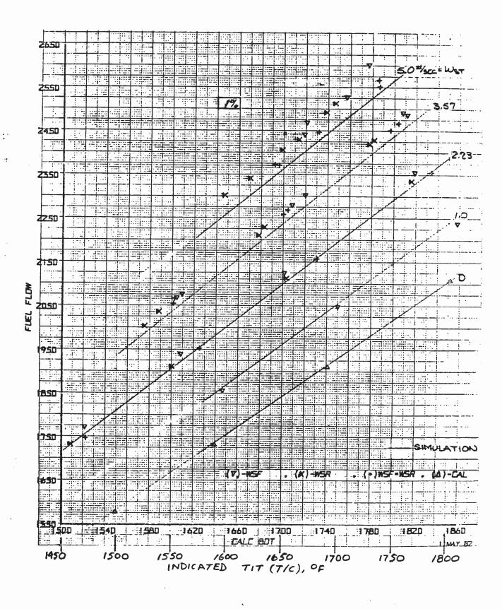
Figure 4 501  $^{\circ}$  steam  $^{\circ}$  injection test data -  $W_{f}$  vs calc BOT
