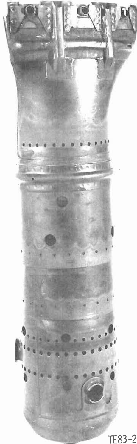
Figure 17. Combustor following DFC testing.
