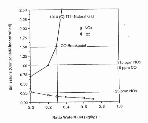
In Figure 4-3, the Cheng Cycle system is operated at the maximum steam injection rate (2.5 kg/sec) with the turbine fired at maximum inlet temperature (1010 degrees C.) on natural gas. Here the water injection CO threshold occurs at about 0.3 kg water per kg fuel, with an associated exhaust NOx reduction of about 85%.
