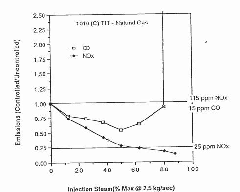
Cheng Cycle intrinsic steam injection can eliminate the need for a water injection control system. For instance, the current Dutch gas turbine NOx emission control standard (135 g/GJ) can be met simply by establishing a minimum steam injection setpoint of about 20% of maximum (natural gas firing). This reduces system installation and maintenance cost and complexity and avoids the increased carbon monoxide and hydrocarbon emissions associated with water injection
