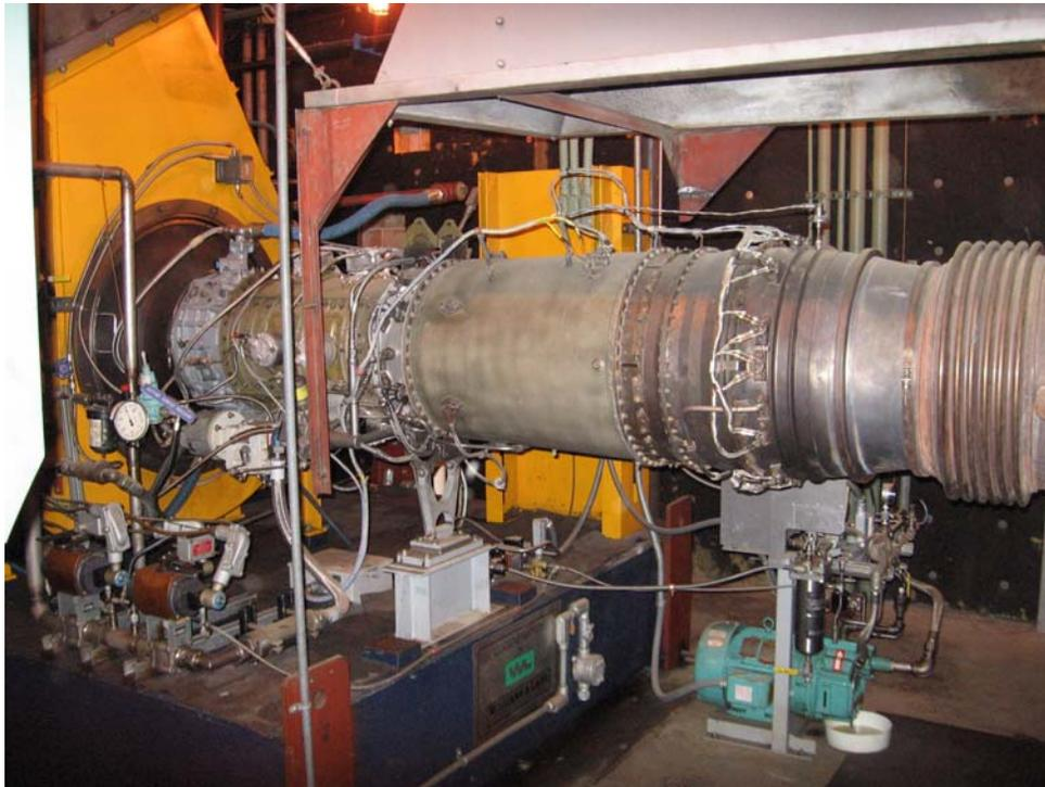
The **Allison 501-KB5S** engine weights approximately 1,300 pounds, is 8 feet in length, has a maximum mechanical limit of 25,000 lb. in. output torque, and operates in a speed range of 12,350 to 14,500 rpm. Engine rotation is counterclockwise as viewed from the exhaust end. The lubrication system includes a main and scavenge oil pump.
